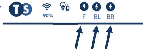
These images appear when sensors are activated (F=Front Sensor, BL=Back Left Sensor, BR: Back Left Sensor). The sign will then dim when any or all these sensors are activated, when app is connected to sign.
